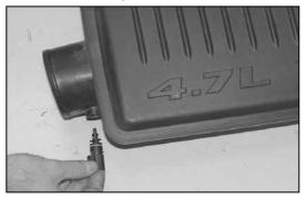
24. Rotate the air temperature sensor counter clockwise and remove the sensor from the stock intake plenum as shown.
