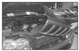
6. Remove the six grill retaining clips from the grill, then tilt the grill forward and lift to remove from the vehicle.
