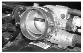
21. Install the silicone hose (084031) onto the throttle body and secure with the provided hose clamp.
