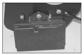
15. Using the provided spacer, install the vacuum reservoir onto the heat shield as shown. NOTE: Due to vehicle manufacturing tolerances, 2 spacers may be required. NOTE: Some vehicles may not be equipped with a vacuum reservoir.
