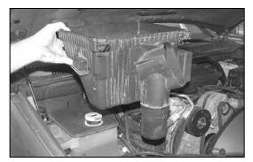
9. Lift the lower airbox and remove it from the vehicle as shown.
