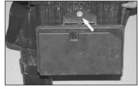
14. Remove the bolt that secures the vacuum reservoir to the airbox and then remove the reservoir from the airbox. NOTE: Some vehicles may not be equipped with a vacuum reservoir.
