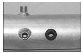
25. Install the supplied rubber grommet into the  $K\&N^{\otimes}$  intake tube as shown.
