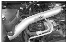
28. Install the K&N<sup>®</sup>intake tube into the silicone hose at the throttle body and align with the tube mounting bracket installed in step #23. Secure with the provided hardware and hose clamp. **NOTE: Due to the different style of A/C lines**
