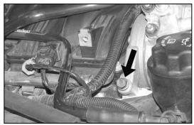
22. Remove the lower rear A/C mounting bolt show. **NOTE: This bolt will be reused.**
