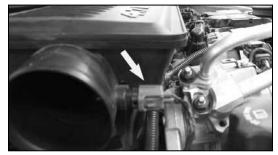
20a. Disconnect the air temperature electrical connection.
