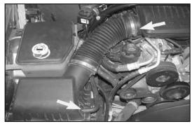
2a. Loosen the hose clamp, which secures the stock intake tube to the intake plenum, and disconnect the crankcase vent hose from the air box lid.
