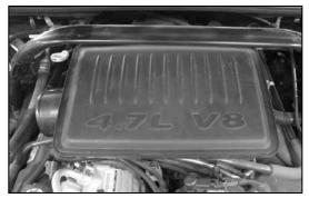
20b. Remove the two bolts that secure the intake plenum to the intake manifold.
