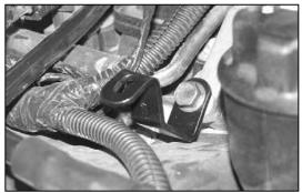
23. Install the tube mounting bracket onto the A/C
