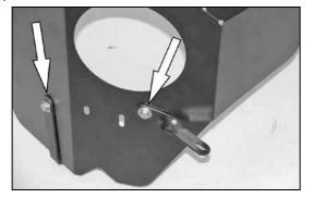
13. Install the Install the heat shield mounting bracket and twist bracket onto the heat shield as shown using the provided hardware.
