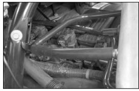
30.Install the supplied silicone hose onto the crankcase vent "T" and connect the other end onto the K&N<sup>®</sup> intake tube as shown.
