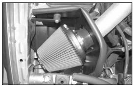
34. Install the air filter assembly onto the K&N<sup>®</sup> intake tube as shown and secure with the provided hose clamp.
